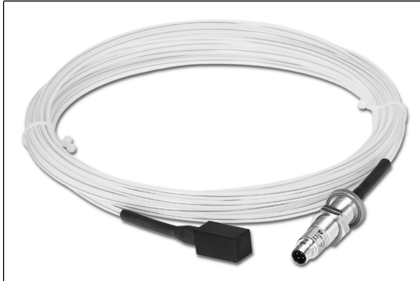
FIGURE 1 – Unibody FOA-100 Fiber Optic Accelerometer with ceramic sensor head, 10-m optical cable, and sealed feedthrough connector with built-in optoelectronic conditioner.
