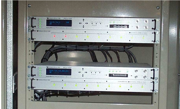
Figure 8: PCU-100 Programmable Monitor Used with FOA Accelerometers
