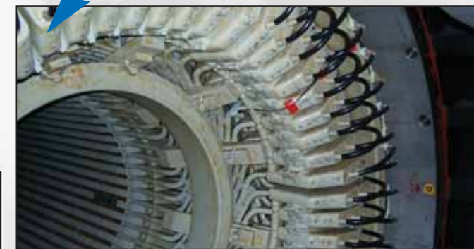
End-winding vibration monitoring on a turbogenerator: helps to prevent deterioration of support and insulation systems
