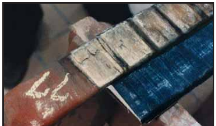
Abrasion of a bar insulation from in-slot vibration (radial) against stator lamination compared to a new bar.
