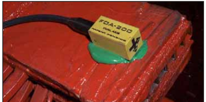
FOA-200, dual-axis, at start of installation procedure. The sensor is being installed on a 540 MW hydrogen-cooled generator.
